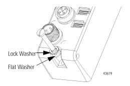
Connect the Input/Output Cord Sets to the ArmorBlock Module The ArmorBlock family offers 5-pin micro-style PCB mounting connectors or 3-pin pico-style PCB mounting connectors.
