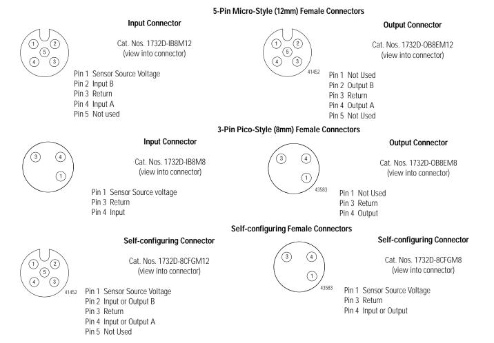
The self-configuring modules (1732D-8CFGM8 and 1732D-8CFGM12) contain both input and output functionality.
