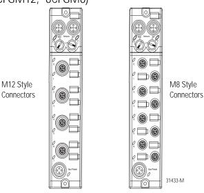
The DeviceNet 1732D ArmorBlock<sup>™</sup> I/O family consists of stand-alone 24V dc I/O modules that communicate via the DeviceNet<sup>™</sup> network. The sealed IP67 housing of these modules requires no enclosure (Note that environmental requirements other than IP67 may require an additional appropriate enclosure.) I/O connectors are sealed M8 (pico) or M12 (micro) styles while the network and auxiliary power connectors are sealed M12 style.
